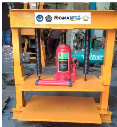
Figure 7. View of Hydraulic Press Machine for Dry Waste Source: processed by the team, 2024
