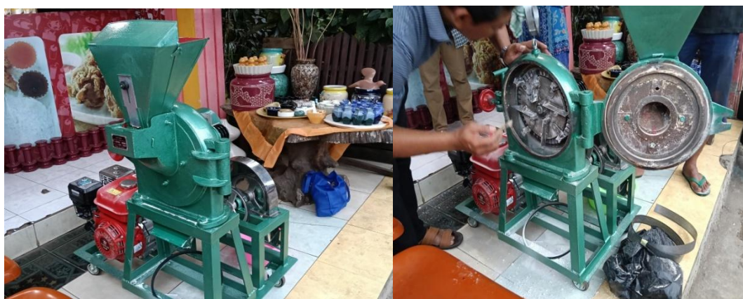
Figure 5. Innovation of Appropriate Technology Biopharmaceutical Grinder Source : Privat Collection
