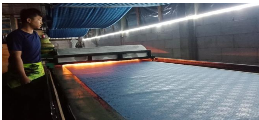
Figure 5. Drying process using gas heating equipment
