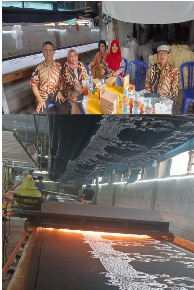
Figure 11. Heating Machine Source: MSME profile (2025)
