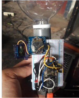
Figure 3. Design of Feeding Equipment and Temperature Monitoring Sumber: Observation results, 2022
