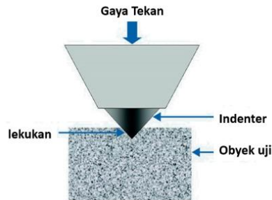
Gambar 1. Prinsip uji kekerasan Rockwell Sumber: Struers Hardness Testing
